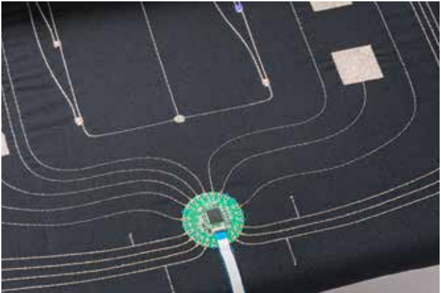
Electronic board placed on fabric and connected with conductive threads.
