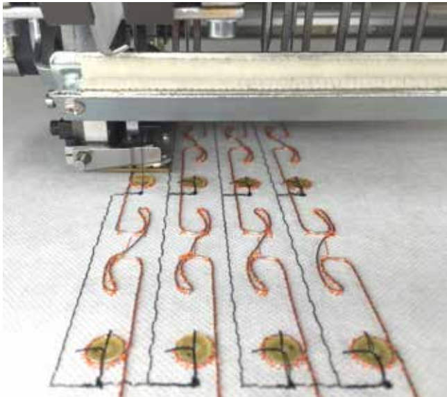
RFID antennas placed and fixed by embroidery.
