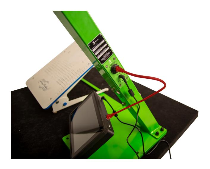
Connect a network cable to the TouchBox and the switch, shown here in red.
